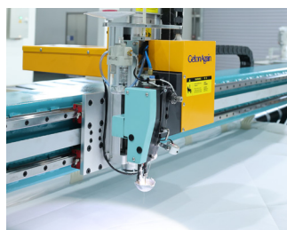
15cm自动升降机头 Lifting sewing head up to 15cm
